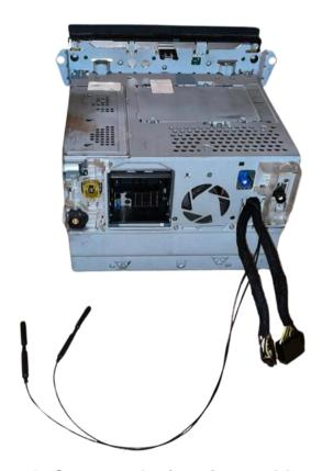
Step 8. Connect the interface cable to the radio (plugs)
