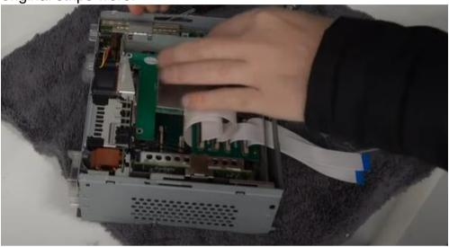
Screw on the new (additional) circuit board.
