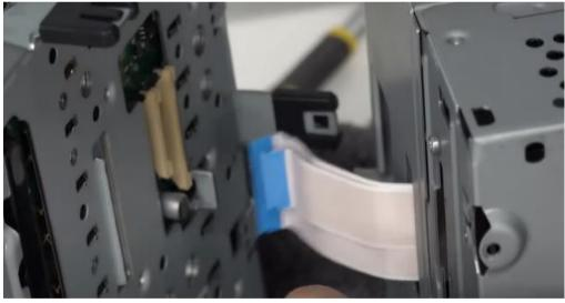
**Step 5. Open up the radio (screws)**Remove the three screws on the back of the radio and slide the lower part back until it comes off .
