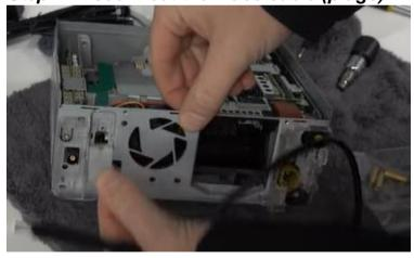
Remove the bracket next to the vent to make room for the passage of the two cables that are clicked onto the circuit board. Position the two antennas as well.
