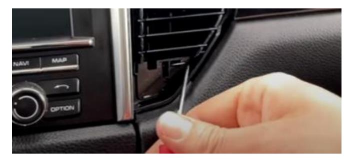
Pull off the right panel using the hook and auxiliary tools. The front panel has one large clip and a number of smaller clips. Press the large clip up slightly from below so that it comes loose.
