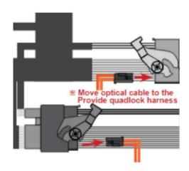
Step 9. Connect the remaining cables to the radio (plugs)
